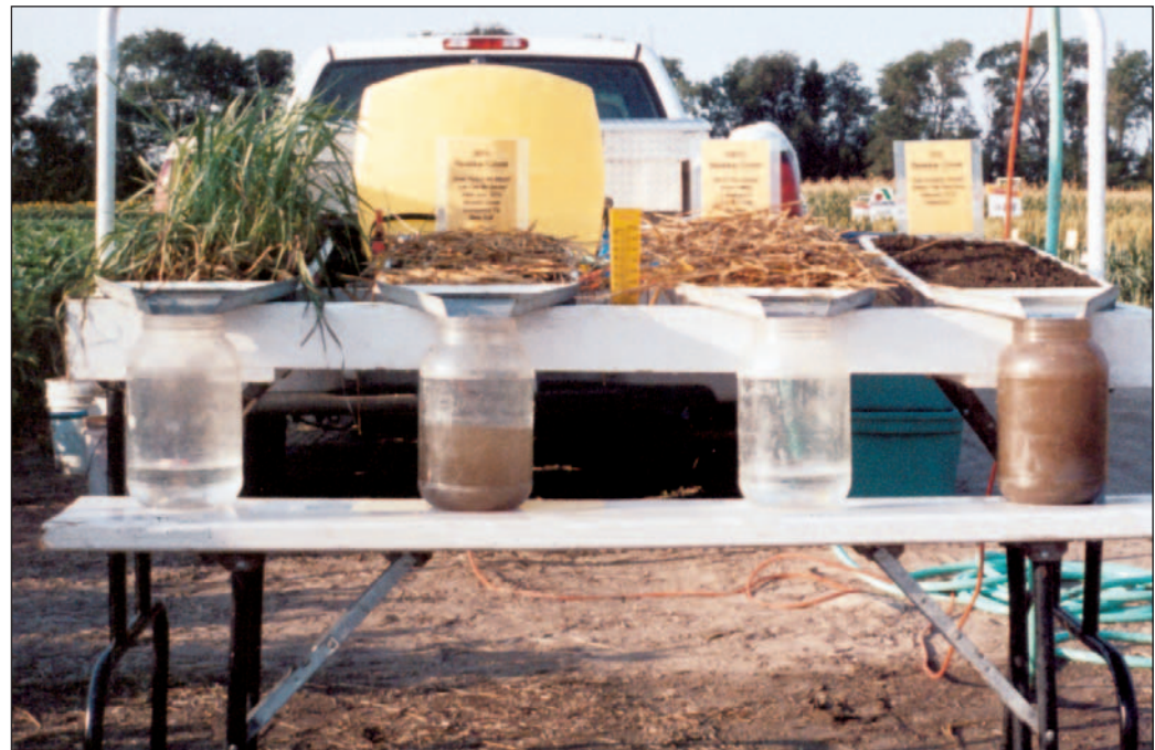
FIGURE 20. This table top rainfall simulator shows the dramatic differences in quantity and quality of runoff associated with high residue farming versus clean tillage. All trays received the same amount of simulated rainfall.
