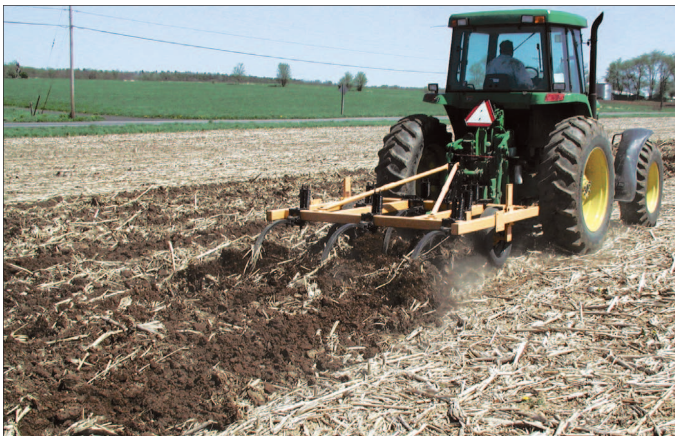
FIGURE 11. Chisel plowing is between moldboard plowing and no-till. It does less soil inversion and leaves more residue cover than the moldboard.
