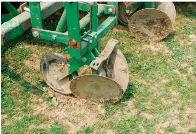
Residue cleaners with concave disks.
