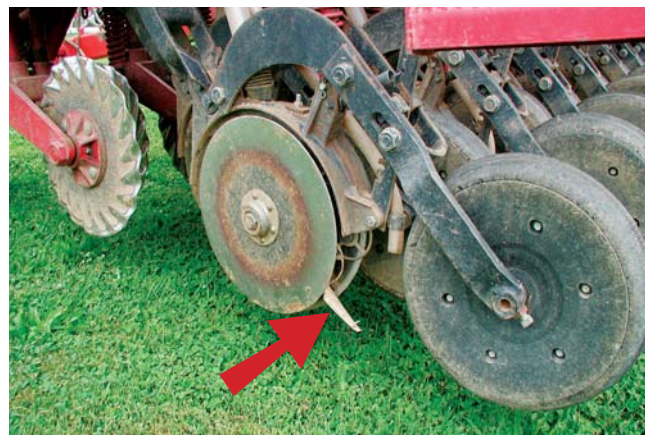
Seed firmer on a drill also pushes the seed into the bottom of the seed slot.
