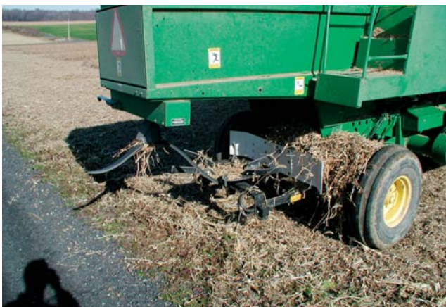
A residue spreader on the combine is essential for successful no-till. Shown are a batt spreader for large residue pieces and a chaff spreader for fine chaff.
