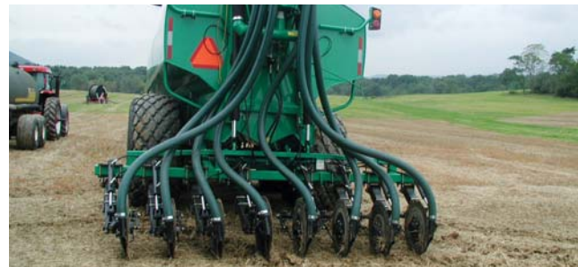
Injection system for liquid manure.
