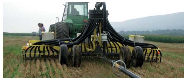
Aerator with manure distribution system and drag hose.
