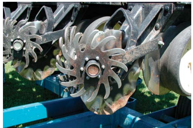
Residue cleaners with curved fingers.
