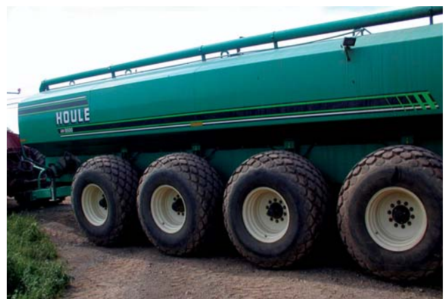
Soil compaction management is necessary in no-till. Using flotation tires helps alleviate surface compaction.
