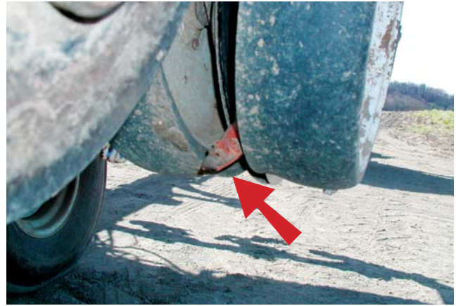
A seed firmer on a planter pushes the seed down into the seed slot to achieve optimum seed depth control. Pop-up fertilizer can be applied through the seed firmer.
