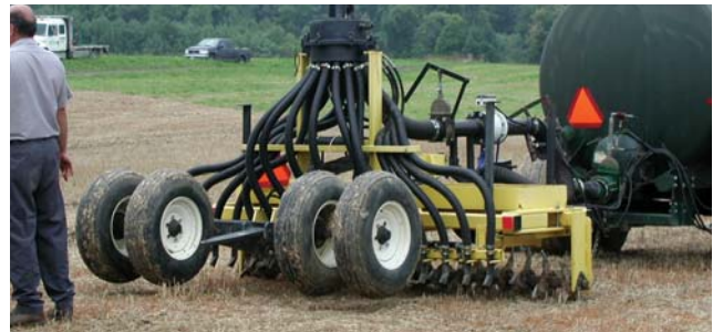
Rotating teeth punch holes in which liquid manure quickly infiltrates.
