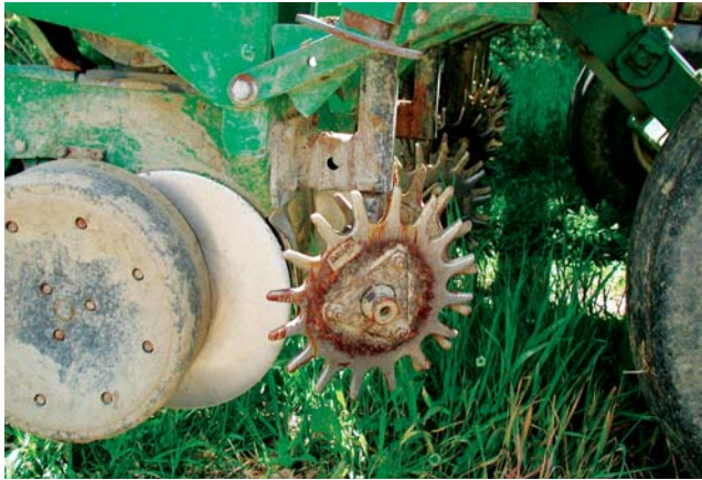
Residue cleaners with straight fingers.
