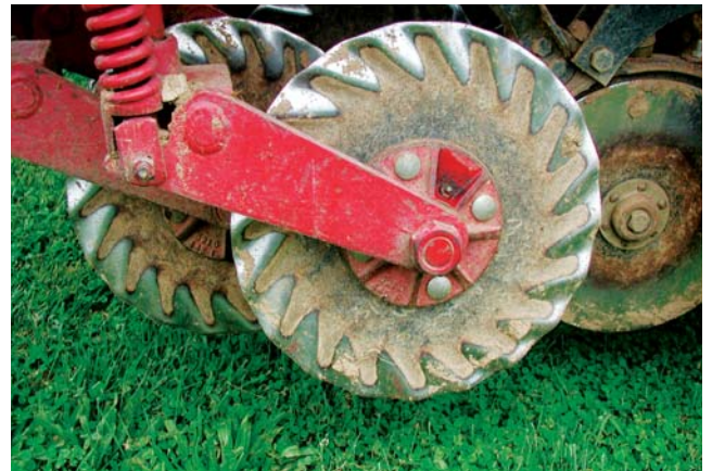
A fluted coulters with angled waves to facilitate soil penetration and reduce soil disturbance.
