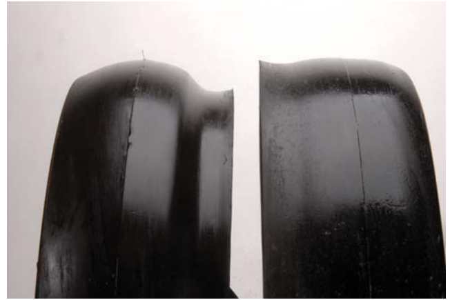
Comparison of two common types of depth gauge wheels. Case IH wheels are on the left and the other commonly used wheel is on the right.
