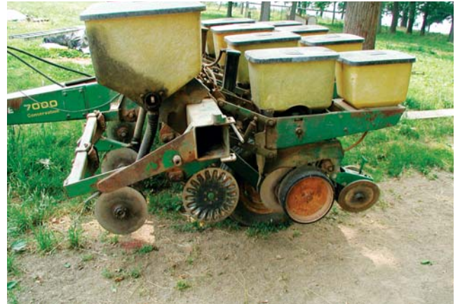
A planter mounted with a bubble coulters.
