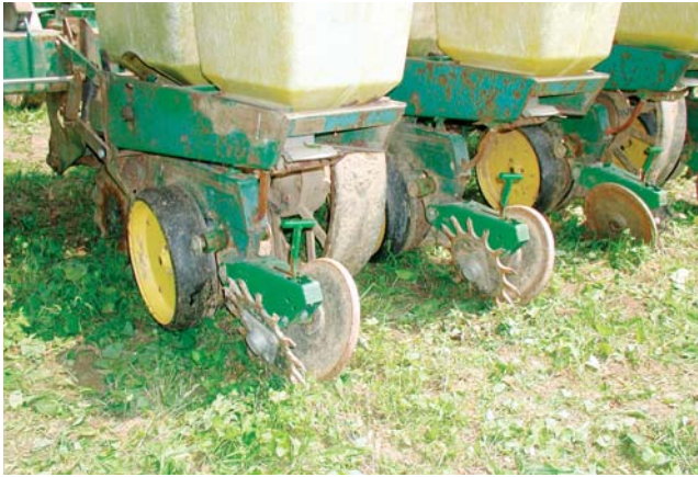
Some farmers mount one fingered and one cast iron closing wheel on a planter unit.
