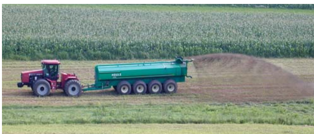
Surface application of liquid manure in no-till.
